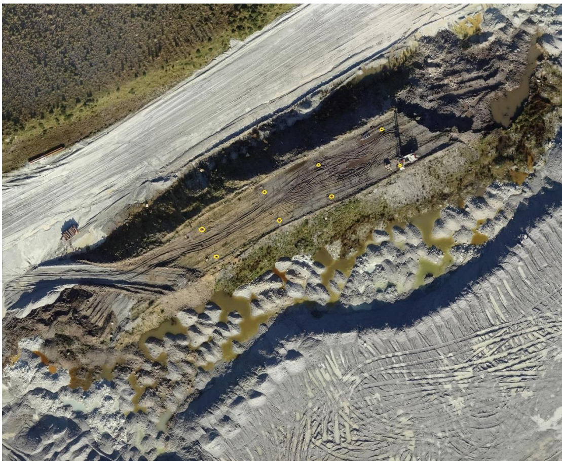
Figure 12: Location of coring samples (yellow circles) on soil tip. Photograph taken Oct 2017 copyright of Sibelco.
