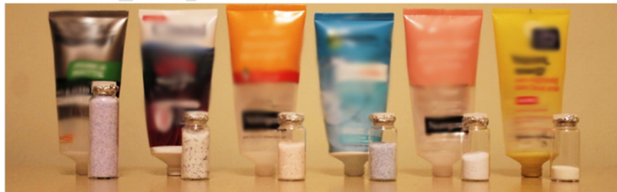
Fig. 1. The samples of microbeads extracted from six different facial products. Photo Credit: Imogen Napper, Plymouth University.
