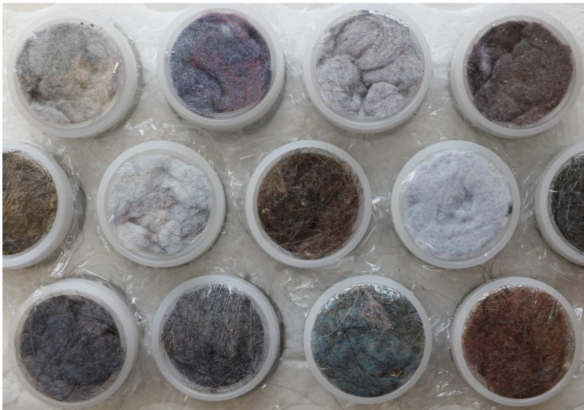
384 Figure 1: A selection of dryer lint samples in 21-mm diameter XRF cups that had been collar-sealed 385 with polyester film.
