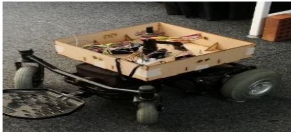
Fig. 3. The autonomous vehicle modified from the mobility scooter
