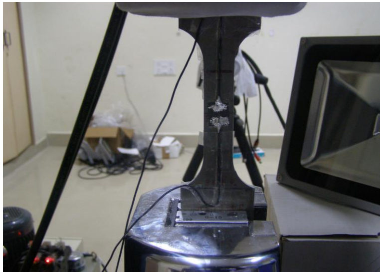
Figure 4: ASTM specimen with nano material based sensor attached at one side
