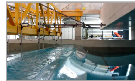
The X-MED buoy moored in the Ocean Basin: being hit by a wave (left) and showing the retroreflective markers used for 3D motion tracking (right).
