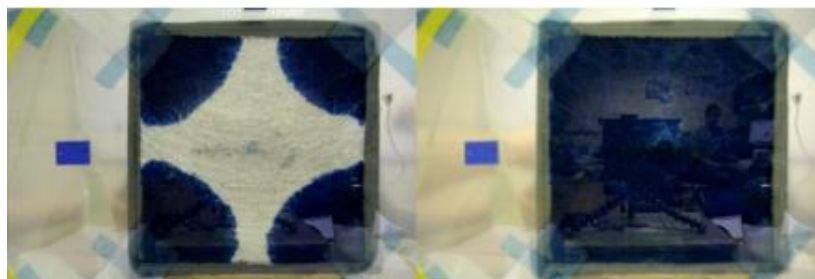
Fig. 5: Comparative stalled flow positions on the reverse face for acrylic (left) and balsa (right) cores.
