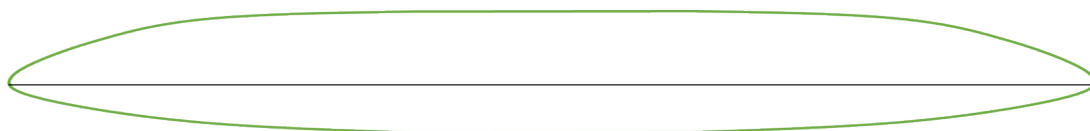
Proposed Spitfire wing tip with small positive pitching moment
