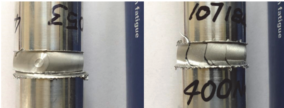
Figure 17: Example of torsion test, T11 ( R=-1 , stress amplitude = 66 MPa) and T16 ( R=0 , stress amplitude = 33 MPa).
