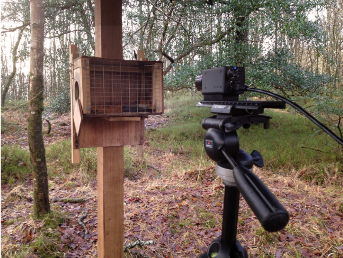
Figure 1. The filming arena. The set-up in the field was designed to attract the birds to the field of view of the camera where a mild acute stressor could be applied, using a feeding box. The set-up consisted of a 25 by 14 cm and 16.5 cm high box built from plywood, with a front panel of galvanized wire mesh with an aperture size of 1 by 2.5 cm. The mesh allows infrared radiation to pass through, making it possible to film birds whilst inside the set-up. Wire mesh was chosen, as glass and most plastics do not transmit infrared radiation. A hole of 60 mm diameter was cut in the left end wall to allow bird entering the set-up and gain access to the food placed at the right end of the box. A temperature logger probe sandwiched between two squares of black insulation tape (marked by black arrow) is attached to the top right corner of the front panel to record a reference temperature. The mild acute stressor is applied to the bird inside by closing the box. Pulling on a fishing line attached to a rotating door at the entrance hole allowed the experimenter to close the box when a bird is inside. The thermal imaging camera set in front of the trap records the whole sequence of events. Please click here to view a larger version of this figure.
