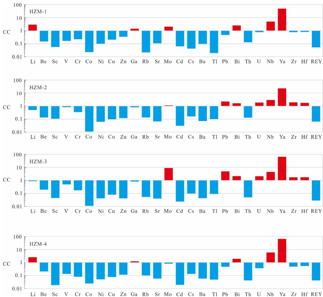
Fig. 12. Concentration coefficients (CC = ratios of element concentration in samples vs world clays, Dai et al., 2015b) of trace elements in tonsteins, normalized by the mean composition of clay shale (Grigor'ev, 2003).
