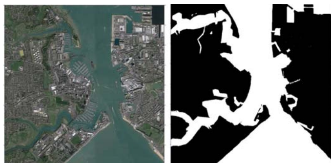
Fig. 2. Satellite image of Portsmouth Harbour and its corresponding binary image (Source: Google Maps)
