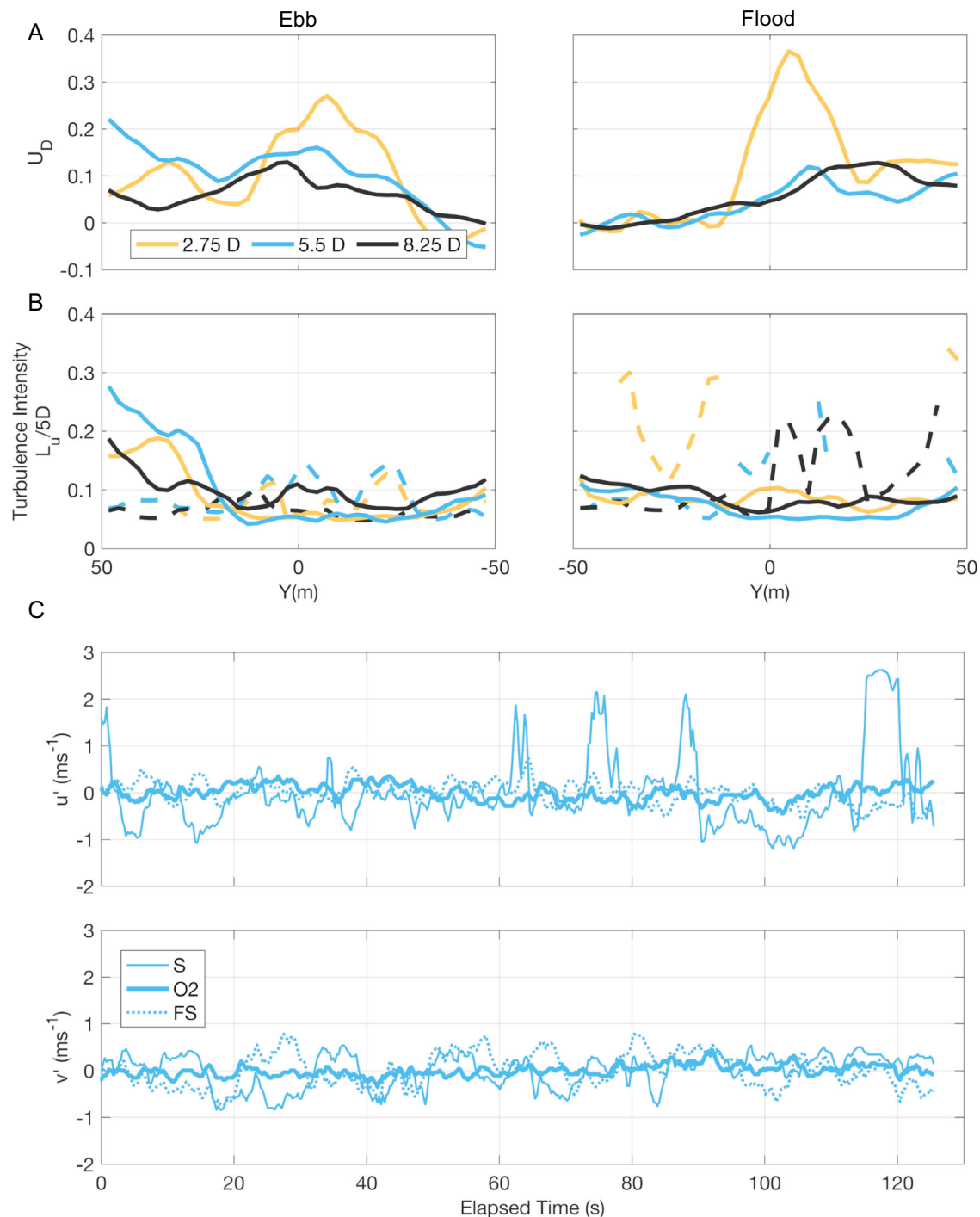
Fig. 8 | PIV-derived surface wake velocity deficit and turbulence characteristics as a function of downstream distance and surface velocities comparing the O2's wake with the adjacent natural flows. A, B Peak ebb (left, 17/04/2022, T6, 3.2 \text{ ms}^{-1} ) and flood (right, 17/04/2022, T1, 3.2 \text{ ms}^{-1} ) hovers at different downstream distances indicated by colours. A Streamwise spatially averaged wake velocity deficits ( U_D ). B Streamwise spatially averaged turbulence intensity (lines) and
