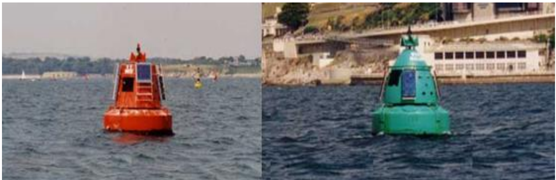
Figure 3-4: Navigation channel marking buoys in IALA A region; where the port buoy is red can-shaped while the starboard buoy is green cone-shaped
