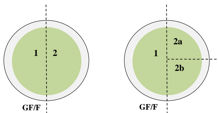
Figure 3.1. Schematic of filter portioning for samples collected on the Arctic ICE project 2011. 1 and 2 represent portioning in two halves whilst 2a and 2b represent portioning in quarters (Filter size 47mm).
